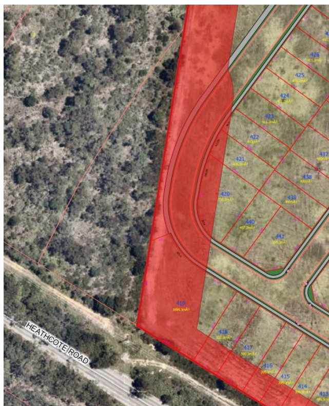
Figure 05: Additional APZ setbacks if a downslope was taken as the effect slope towards the allotments.
